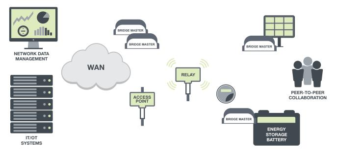
The Relay 5 in conjunction with the AP 5 extends the speed and coverage of the network to deliver high-capacity data securely and reliably from the edge devices to a variety of IT/OT systems.
