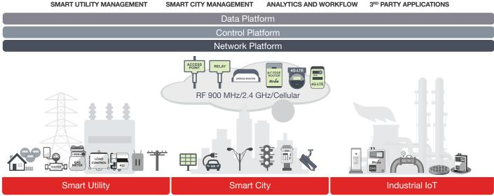
Itron's Gen5 solution supports a range of smart grid applications on a single open standards-based network.
