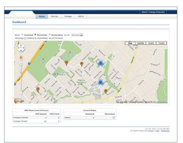
ODS processes last gasp and restoration data arriving from the AMI network and displays this information on a map allowing utility staff to see the extent of an outage.
