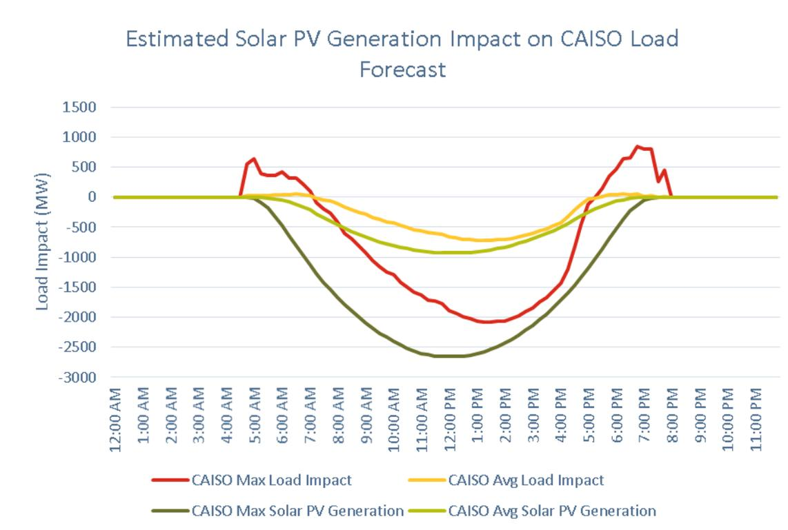
**Figure 51: Estimated Load Impact of Solar PV Generation: PG&E Total**
