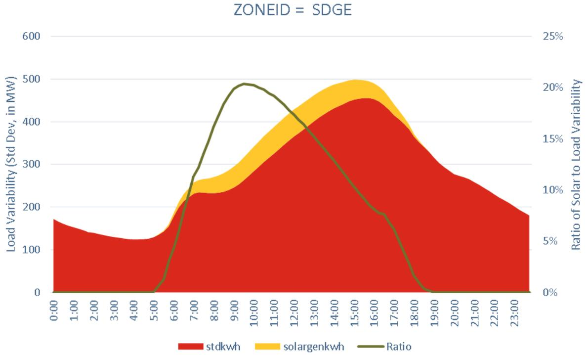
**Figure 4: Ratio of Solar Generation Volatility to Load Volatility: IOU Comparison**
